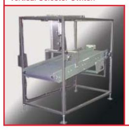
Our Vertical Selector Switch is used to switch Pans, Lids, Trays, Baskets or Products from one Conveyor Line into two or three superposed (same vertical plane) receiving lines. This type of switch is generally used when the selection of the receiving conveyor lines is made prior to the start-up of the production, generally the switching is not possible while running.
